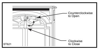
Fig. 28 To open the front doors, turn handle counterclockwise.
